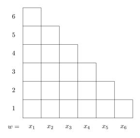
Each entry M[i,j] will contain the set of variables that can generate the substring  $x_j x_{j+1} \cdots x_{i+j-1}$  of w. Note that the row number corresponds to the length of the substring.
